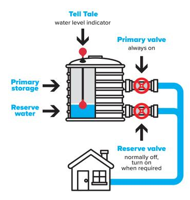
Tanks should be set-up to allow for a minimum reserve storage of one quarter of the capacity, to cover one day's allocation and keep a household functioning for a day. The portioning of storage needs to be controlled by valves (see diagram). Under normal use, the upper valve (Primary) would be on. The lower valve (Reserve) would normally be off, and only opened when required.
